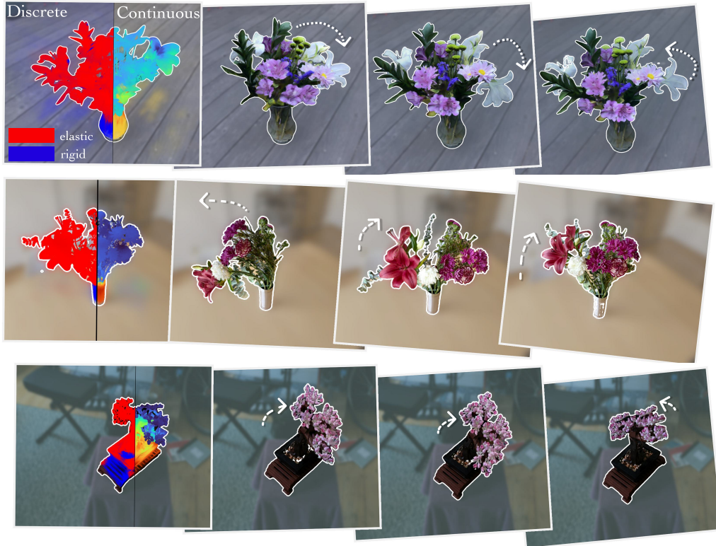
Figure 7: SUPPHYSFIELD’s Zero-shot Real-scene Generalization. Trained only on synthetic SUPPHYSVERSE, SUPPHYSFIELD can predict plausible physic properties, enabling realistic MPM simulation of real scenes. Here, we visualize the material types (left) and Young’s modulus (right) prediction in the first frame, and subsequent frames impacted by a wind force. Please see the videos in our website https://neurips-2025-20627.github.io/ .
